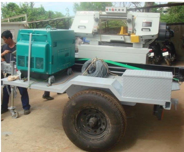
Trailer fitted with remote controlled bomb cutting equipment
